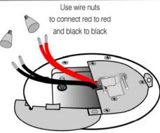
NOTE: Remove 2 screws securing strain-relief clamp and replace with listed conduit connector when conduit connection is required by local codes.
