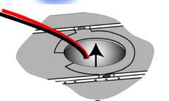
(a) Insert and center the speaker into the ceiling opening. Make sure all four doglegs rest on the Cring. (b) Tighten down the four doglegs by turning the screws,located on the driver side of the baffle,clockwise.
